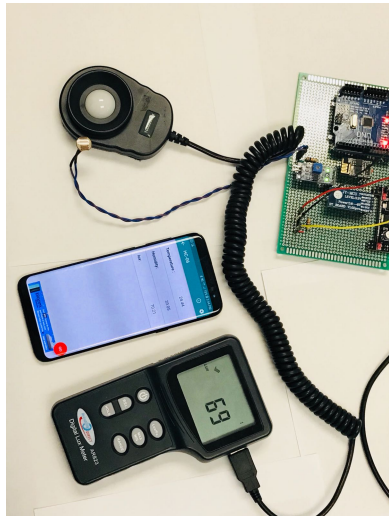
Figure 14: Setting used to test Photo resistor
