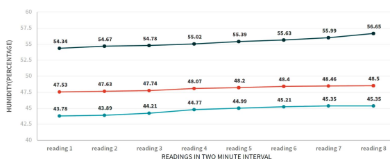
Figure 10: Graph showing the variation in humidity when wet sample is used
