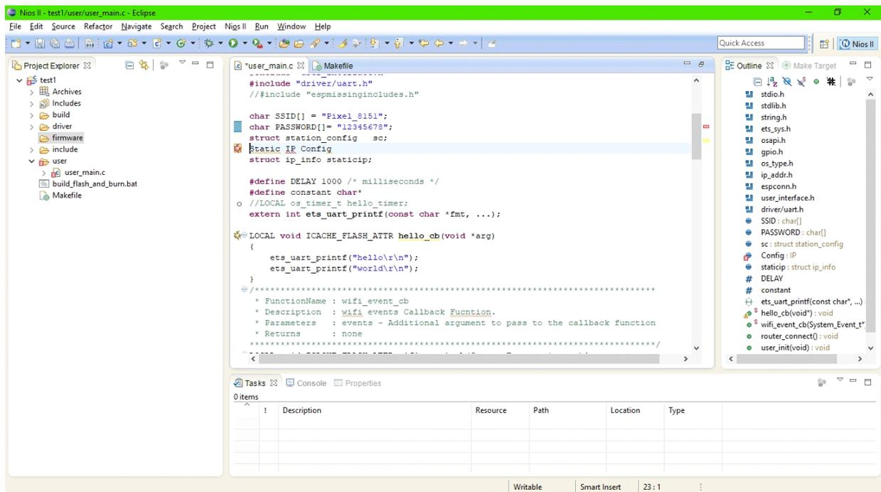
We included all the header files that was in the sample program for the “hello\_world”. Then SSID and password is declared as character arrays. The ESP8266 is configured in station mode and is given a static IP. The linker to store the instructions in flash memory is also declared.
