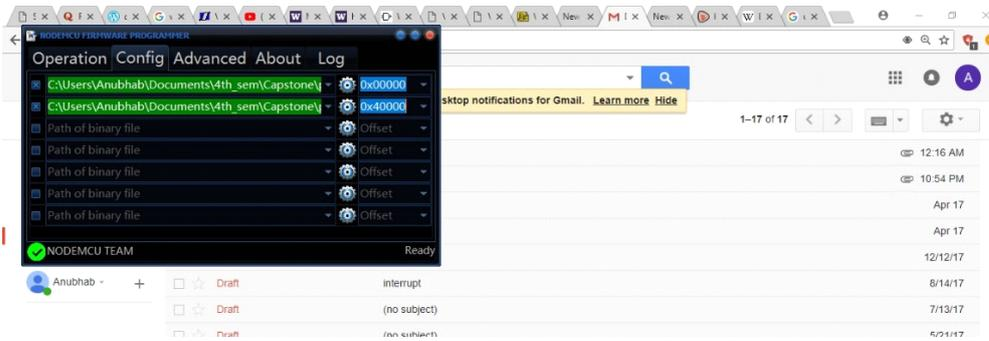
After solving the error we again re-built the project in Eclipse and it got built without any errors. Then we used the ESP Flashing Tool to flash the firmware onto the ESP8266 module.
