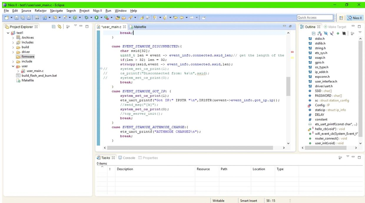
We have created a function called `wifi_event_cb()` which has the event as its parameter. We have used switch-case statement to check the if the device is connected on the network, is disconnected from the network, if the ESP received the IP of the local network which acts as the Master in this configuration and to check if the authentication has changed.
