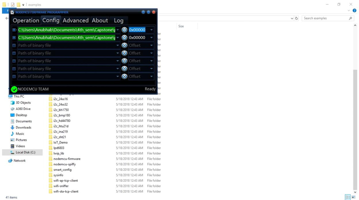
Then we discovered while looking at the makefile that the memory address for the two binary files are provided inside the makefile.
