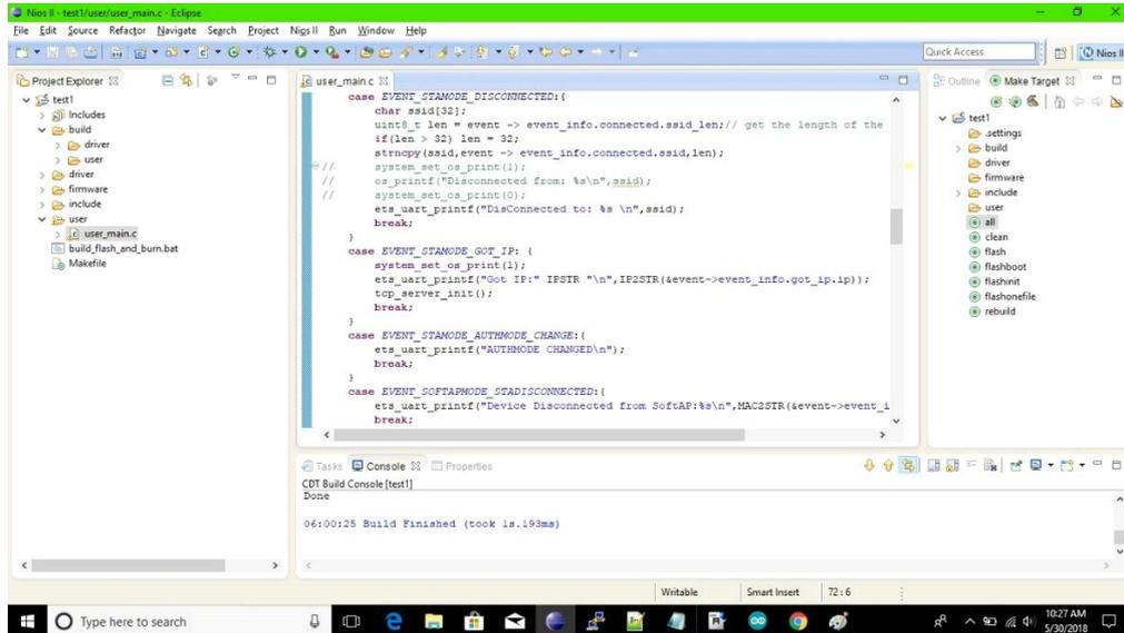
After this we started writing the code to configure the TCP\_IP port of the ESP-8266. The ESP-8266 has five TCP\_IP port for communication between the host and the client. It has got five ports for communication out of which I will be using four ports for the time being. We wrote the local function `LOCAL void ICACHE_FLASH_ATTR tcp_server_init()` in which we setup the TCP\_IP as following:
