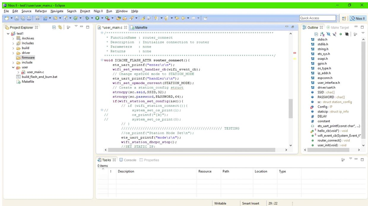
We wrote a function called `router_connect()` to initialize connection to the router. The SSID and Password that was defined above is used to connect to the wifi network. Then the IP, Gateway and net mask are set for the ESP8266 to connect to the router.
