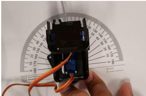
Figure 8: Motor Directed toward 90 Degree
